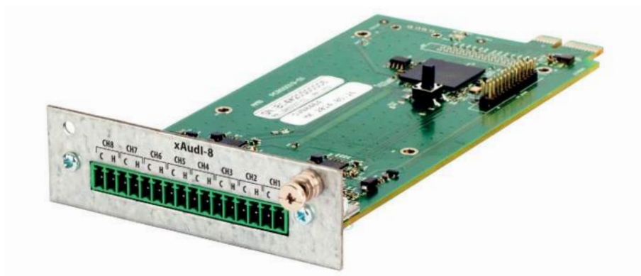
Drawing 29. 8 audio input card
