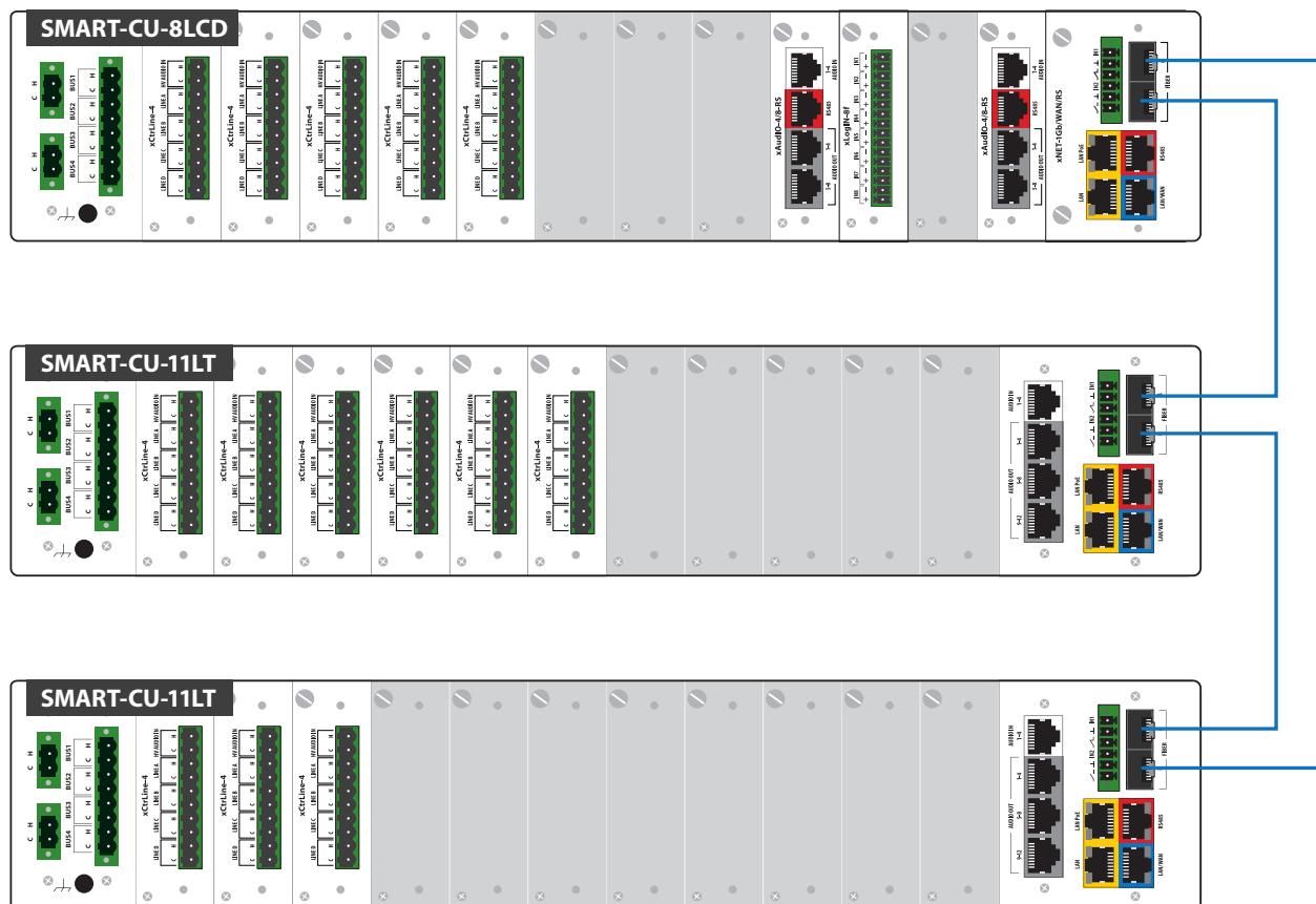
Drawing 73. Connection of control units in Ring topology (optical fibre)
